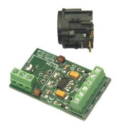
Both balanced input signals are buffered by very high quality Opamps, both present in the THAT128x IC. Besides these opamps there are also 8 laser trimmed resistors in the IC.
